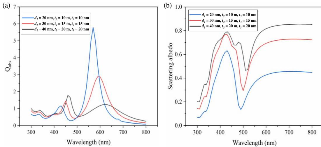
**Fig. 5** Effects of nanoparticle sizes on (a) absorption efficiency and (b) scattering albedo of the Ag-SiO<sub>2</sub>-Ag composite nanoparticle.
