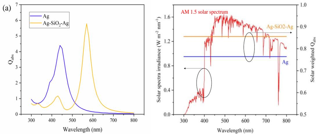
**Fig. 2** Comparison of (a) absorption efficiency, (b) Solar weighted absorption efficiency of Ag and Ag-SiO<sub>2</sub>-Ag [right axis], and the AM 1.5 solar spectral irradiance applied as the spectral weights [left axis].
