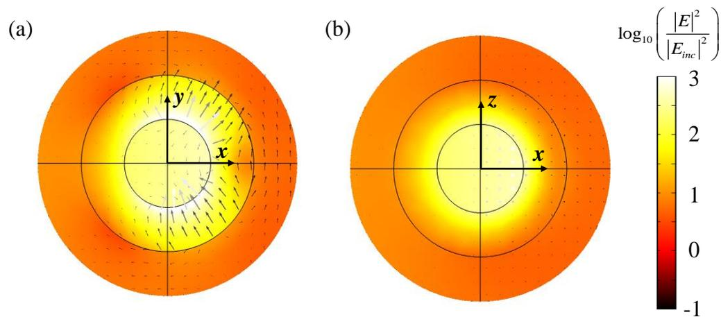
**Fig. 4** Local field distribution at the wavelength of 430 nm for the Ag-SiO<sub>2</sub>-Ag composite nanoparticle when the applied plane wave is  $x$ -incidence and  $y$ -polarization. The arrows indicate the electric field vector when the phase = 0 degrees.
