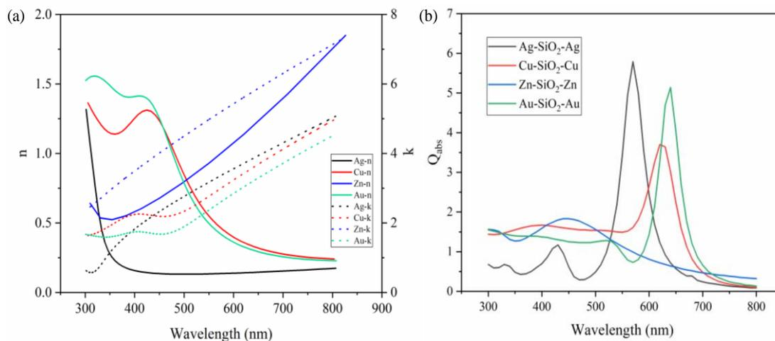
**Fig. 6** (a) The real and imaginary parts of the complex refractive index, *i.e.*,  $n$  and  $k$  respectively, for the four metals, Ag, Cu, Zn, and Au.<sup>[44]</sup> (b) Effect of different metal materials on the absorption efficiency for the metal-insulator-metal composite nanoparticle. The sizes remain as  $d_1 = 20$  nm,  $t_2 = 10$  nm and  $t_3 = 10$  nm.
