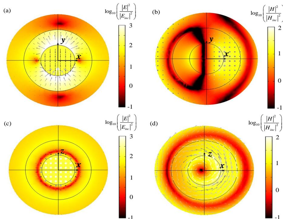
**Fig. 3** Local field distribution at a wavelength of 570 nm for the Ag-SiO<sub>2</sub>-Ag composite nanoparticle when the applied plane wave is *x*-incidence and *y*-polarization. Time-averaged square of (a) the electric field and (b) magnetic field distribution in the *x-o-y* plane; (c) the electric field and (d) magnetic field distribution in the *x-o-z* plane. The arrows denote the electric field vectors in Fig. 3(a), (c), and magnetic vectors in Fig. 3(b), (d) when the phase = 0 degrees.
