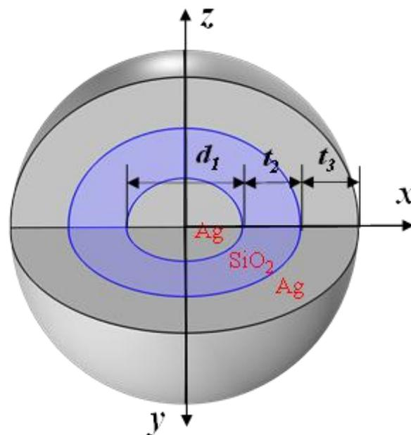
**Fig. 1** Schematic of the proposed core/shell/shell shape Ag-SiO<sub>2</sub>-Ag composite nanoparticle, with  $d_1 = 20$  nm,  $t_2 = 10$  nm, and  $t_3 = 10$  nm.
