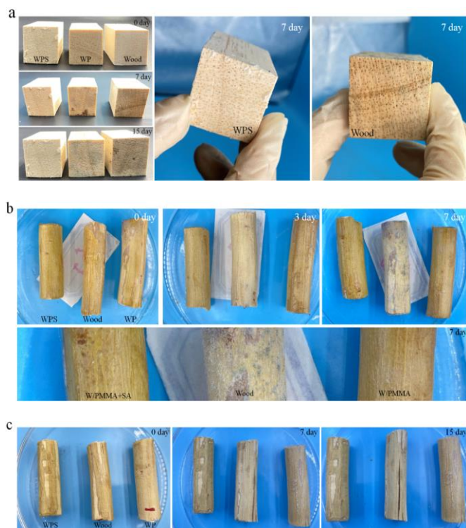
Fig. 4 Characterization of anti-mold and anti-cracking properties of composite wood materials. (a) Digital photos of the balsa-based composite wood after being placed at 25 °C for 15 days; (b) Digital photos of the willow-based composite wood after being placed at 25 °C for 7 days; (c) Cracking resistance of willow-based composites during high-low temperature cycling. Note: Composite wood was placed at 25 °C for 12 hours during a relative humidity of 90%, and then transferred to an environment of 80 °C for 12 hours.
