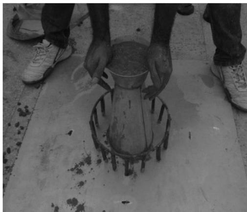
Fig. 4 Illustration of the slump and J-ring test.
