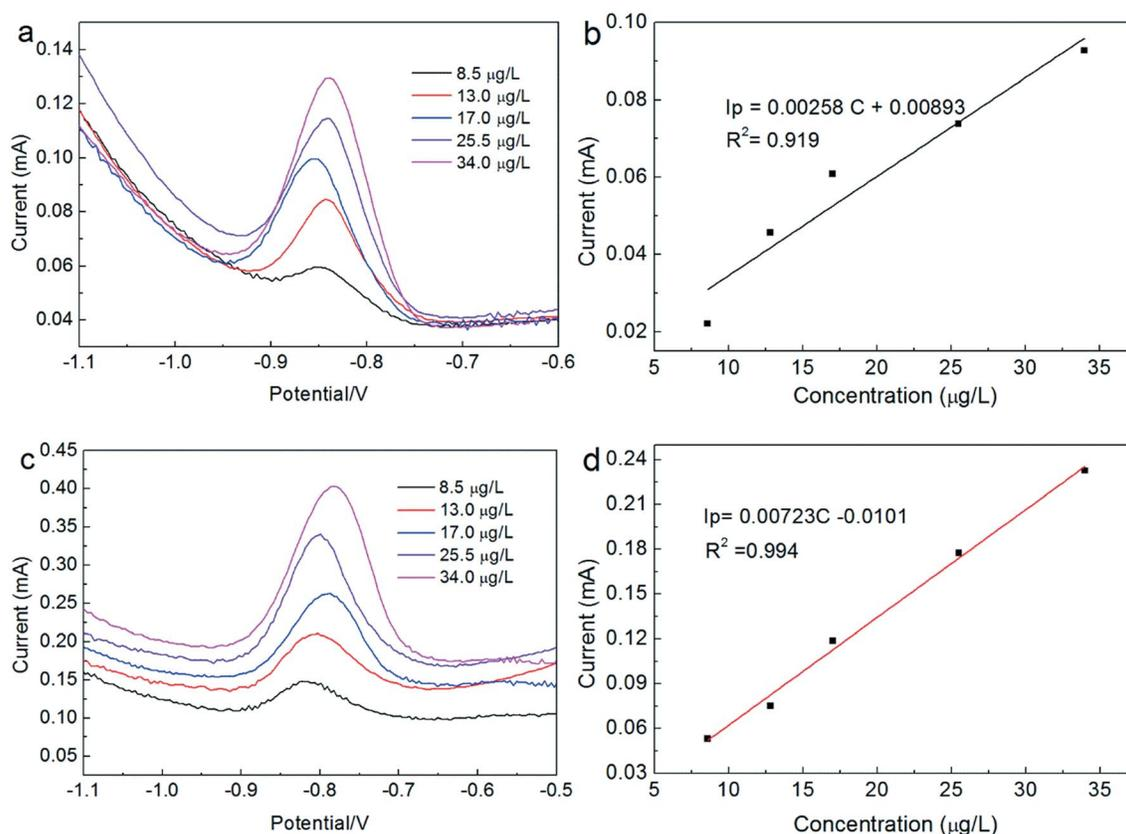
**Fig. 5** SWSV curves of CP (a) and BiMOF/CP (c) with different concentrations of  $\text{Cd}^{2+}$  in the range from 8.5 to 34  $\mu\text{g/L}$ , and the plots of stripping peak current vs.  $\text{Cd}^{2+}$  concentration for CP (b) and BiMOF/CP (d).
