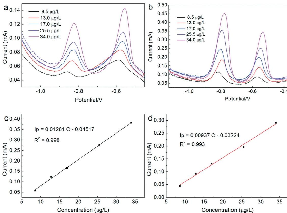
**Fig. 7** SWSV curves for CP (a) and BiMOF/CP (b) with different concentrations of  $Cd^{2+}$  and  $Pb^{2+}$ , and the plots of stripping peak current vs.  $Cd^{2+}$  concentration (c) and  $Pb^{2+}$  concentration (d).
