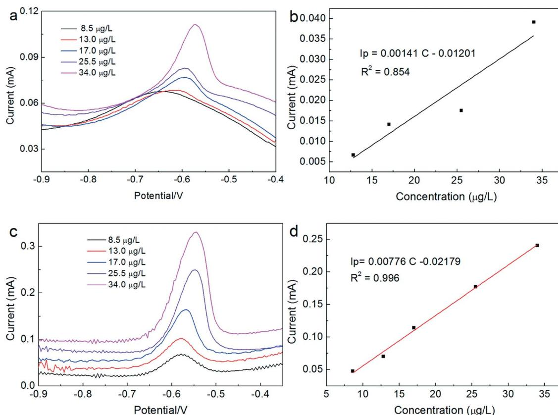
**Fig. 6** SWSV curves of CP (a) and BiMOF/CP (c) with different concentrations of  $\text{Pb}^{2+}$  in the range from 8.5 to 34  $\mu\text{g/L}$ , and the plots of stripping peak current vs.  $\text{Pb}^{2+}$  concentration for CP (b) and BiMOF/CP (d).
