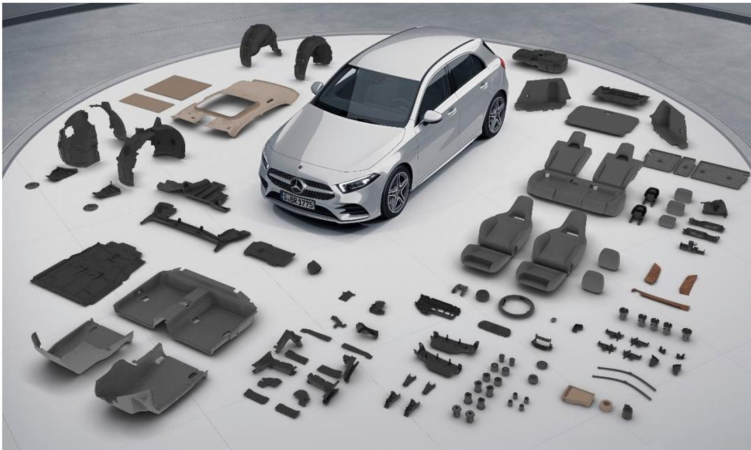
**Fig. 1** New Mercedes-Benz A-Class and its parts made of natural fiber composites. Adapted from Daimler AG, 2018. Reproduced with the permission form [49]. Copyright@Scientific Electronic Library Online.
