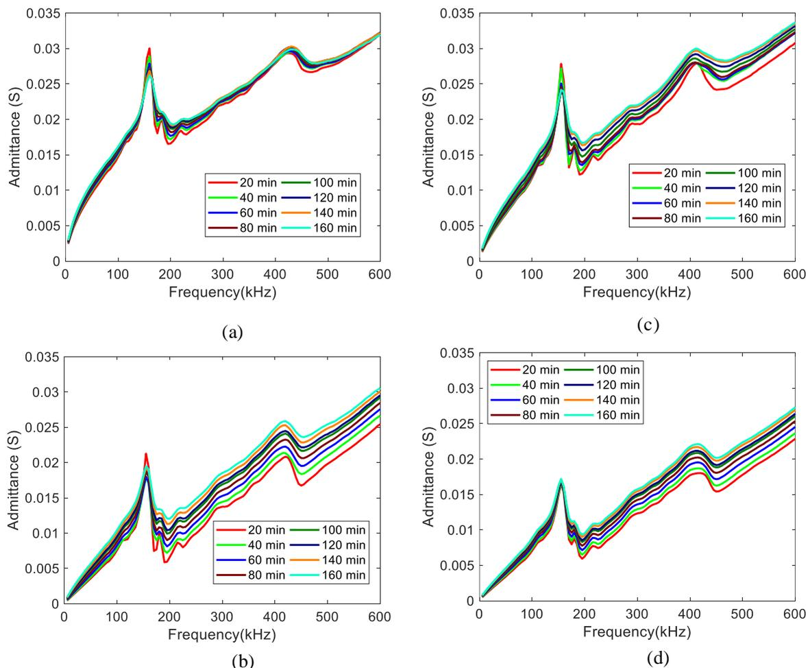
**Fig. 5** EMI spectrum of the sensor embedded in the cement paste with different W/C. (a) W/C=0.3. (b) W/C = 0.4. (c) W/C = 0.5. (d) W/C = 0.6.
