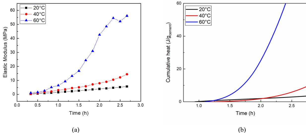
**Fig. 4** Cement pastes with different curing temperatures. a) Elastic modulus results; b) Calorimetric results.
