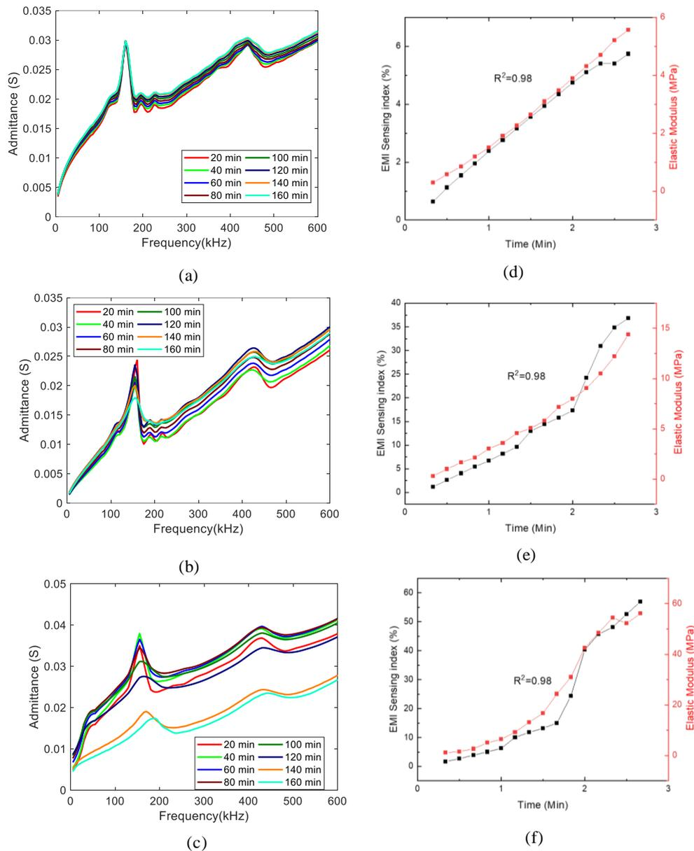
**Fig. 7** Sensing performance of the sensor embedded in the cement paste with different curing temperature. EMI spectrum of cement paste curing at (a) 20 °C, (b) 40 °C, (c) 60 °C. Linear correlation fitting between elastic modulus with EMI-RMSD index for the cement paste curing at (d) 20 °C, (e) 40 °C, (f) 60 °C.
