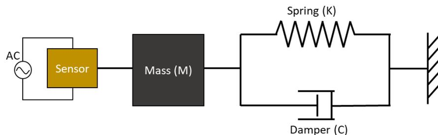
Fig. 2 One-dimension model for piezoelectric sensor-driven structural dynamic system.
