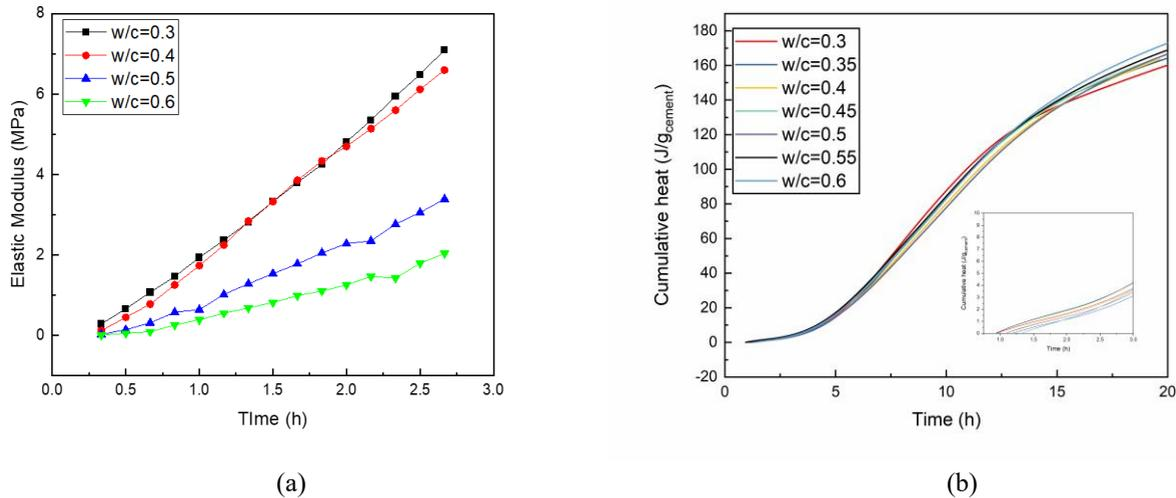
**Fig. 3** Cement pastes with different W/C ratios. a) Elastic modulus results; b) Calorimetric results.
