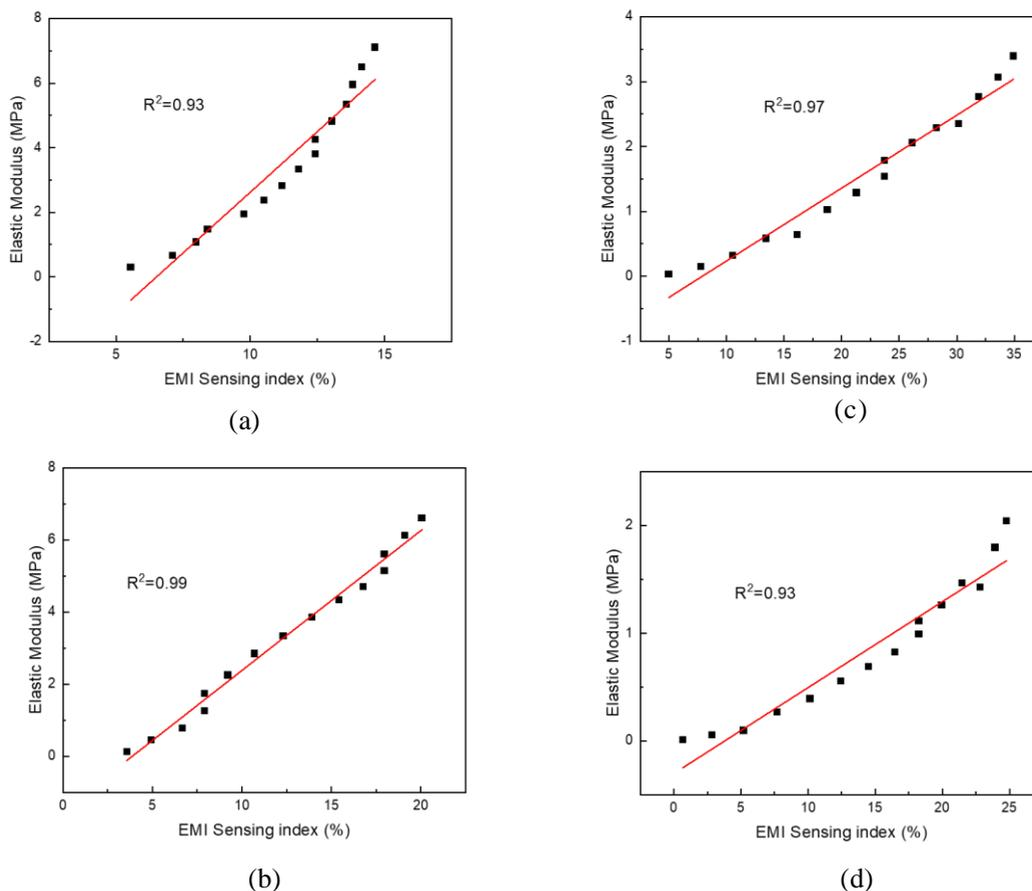
**Fig. 6** Linear correlation fitting between elastic modulus with EMI-RMSD index for the cement paste with different W/C. (a) W/C=0.3. (b) W/C = 0.4. (c) W/C = 0.5. (d) W/C = 0.6.
