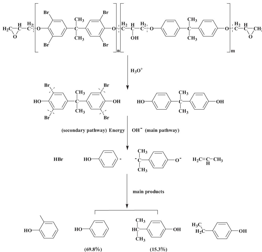
**Fig. 5** A probable decomposition mechanism of BERs during NCW treatment condition.
