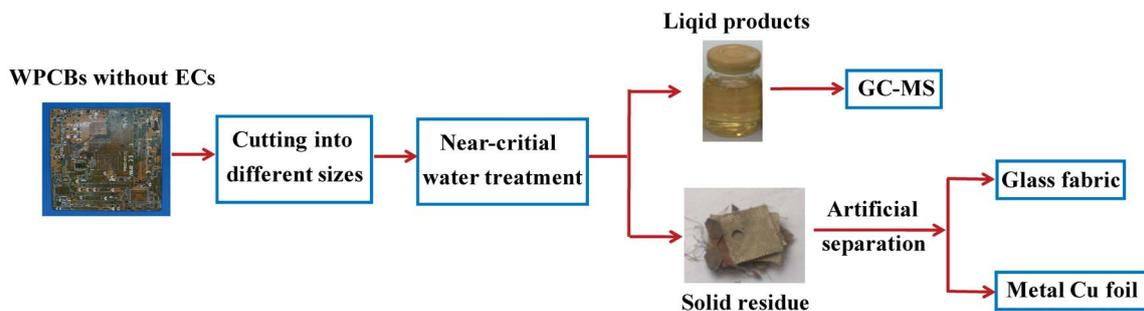
**Fig. 1** The schematic diagram of valuable materials recovery process.
