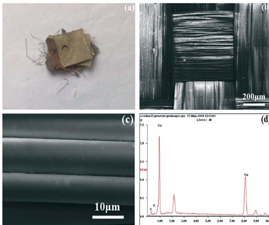
**Fig. 6** The characterization of recovery solid residue: (a) the photograph of recovery glass fabric and metal copper foil, (b) and (c) SEM of glass fabric surface (d) EDS spectrum of copper foil.
