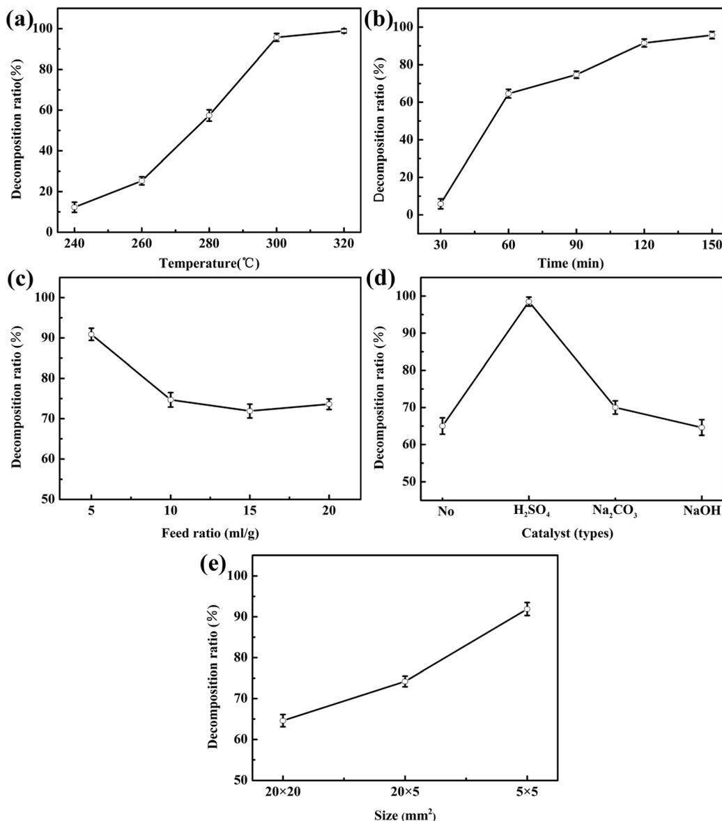
Fig. 4 Effects of various parameters on decomposition ratio of BERs: (a) temperature, (b) reaction time, (c) feed ratio, (d) acid-base type and (e) size of sample.
