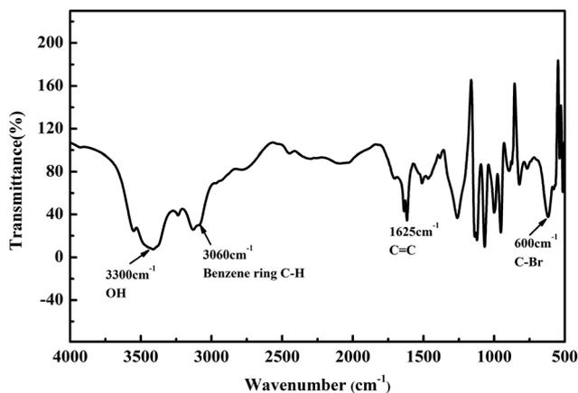
Fig. 3 The FT-IR spectrum of resin matrix in WPCBs.
