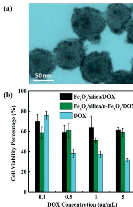
Fig. 7 (a) TEM image of DOX conjugated Fe<sub>3</sub>O<sub>4</sub>/silica/u-Fe<sub>3</sub>O<sub>4</sub> nanoparticles after the electromagnetic triggered release. (b) Cell viability percentage after 48 hrs incubation with Fe<sub>3</sub>O<sub>4</sub>/silica nanoparticles and DOX conjugated Fe<sub>3</sub>O<sub>4</sub>/silica/u-Fe<sub>3</sub>O<sub>4</sub> nanoparticles, and free DOX with various concentrations.
