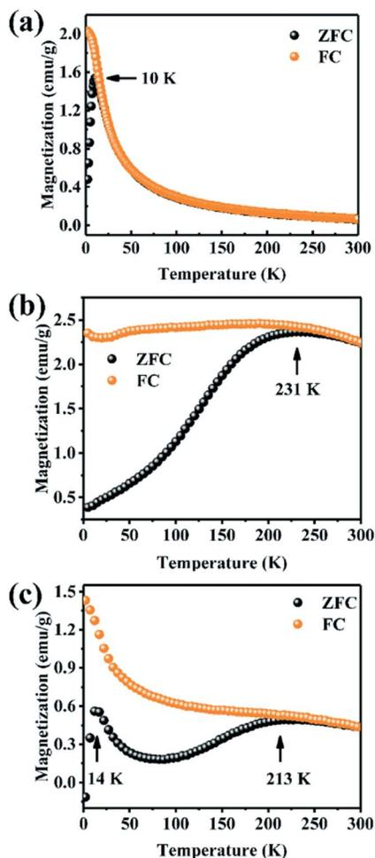
Fig. 4 ZFC-FC curves of (a) ultrathin  $\text{Fe}_3\text{O}_4$  nanoparticles; (b) core/shell  $\text{Fe}_3\text{O}_4/\text{silica}$  nanoparticles; (c)  $\text{DOX}$  conjugated  $\text{Fe}_3\text{O}_4/\text{silica}/\text{u-Fe}_3\text{O}_4$  nanoparticles.
