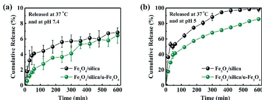
Fig. 5  $\text{DOX}$  release curves of two kinds of nanoparticles, (a) 37 °C, pH 7.4; (b) 37 °C, pH 5.
