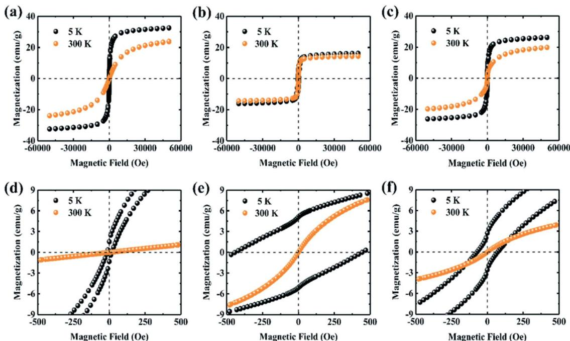
Fig. 3 Magnetic loops of (a) and (d) ultrathin Fe<sub>3</sub>O<sub>4</sub> nanoparticles; (b) and (e) core/shell Fe<sub>3</sub>O<sub>4</sub>/silica nanoparticles; (c) and (f) DOX conjugated Fe<sub>3</sub>O<sub>4</sub>/silica/u-Fe<sub>3</sub>O<sub>4</sub> nanoparticles.
