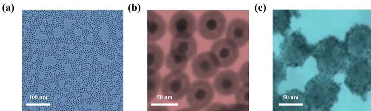
Fig. 2 TEM images of (a) ultrathin Fe<sub>3</sub>O<sub>4</sub> nanoparticles; (b) Fe<sub>3</sub>O<sub>4</sub>/silica nanoparticles; (c) DOX conjugated Fe<sub>3</sub>O<sub>4</sub>/silica/u-Fe<sub>3</sub>O<sub>4</sub> nanoparticles.
