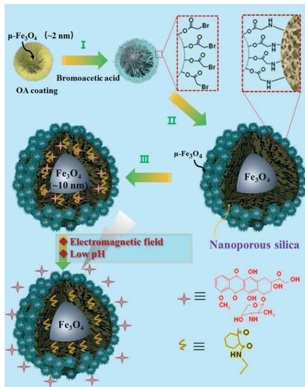
**Fig. 1** Scheme of ultrathin  $\text{Fe}_3\text{O}_4$  nanoparticles decorated  $\text{Fe}_3\text{O}_4/\text{silica}$  nanoparticles for DOX conjugation and release under external pH and electromagnetic field stimuli.
