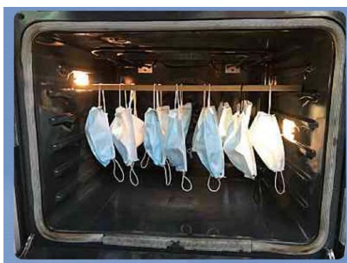
Fig. 4. Suspension of respirators for heat treatment in the oven (Picture provided by Liching Liu).
