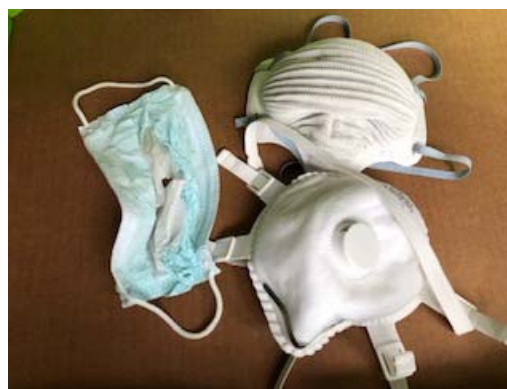
Fig. 5. Breakage of a medical face mask (left) and deformation of two N95 (right) after atmospheric steam treatment for three minutes.
